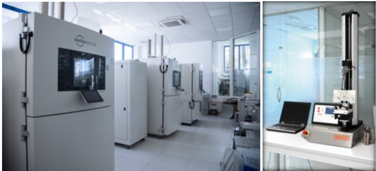
Fig. 32–33 – Aging chambers and Pull & Shear equipment. Source: PreventLab, 2026.
